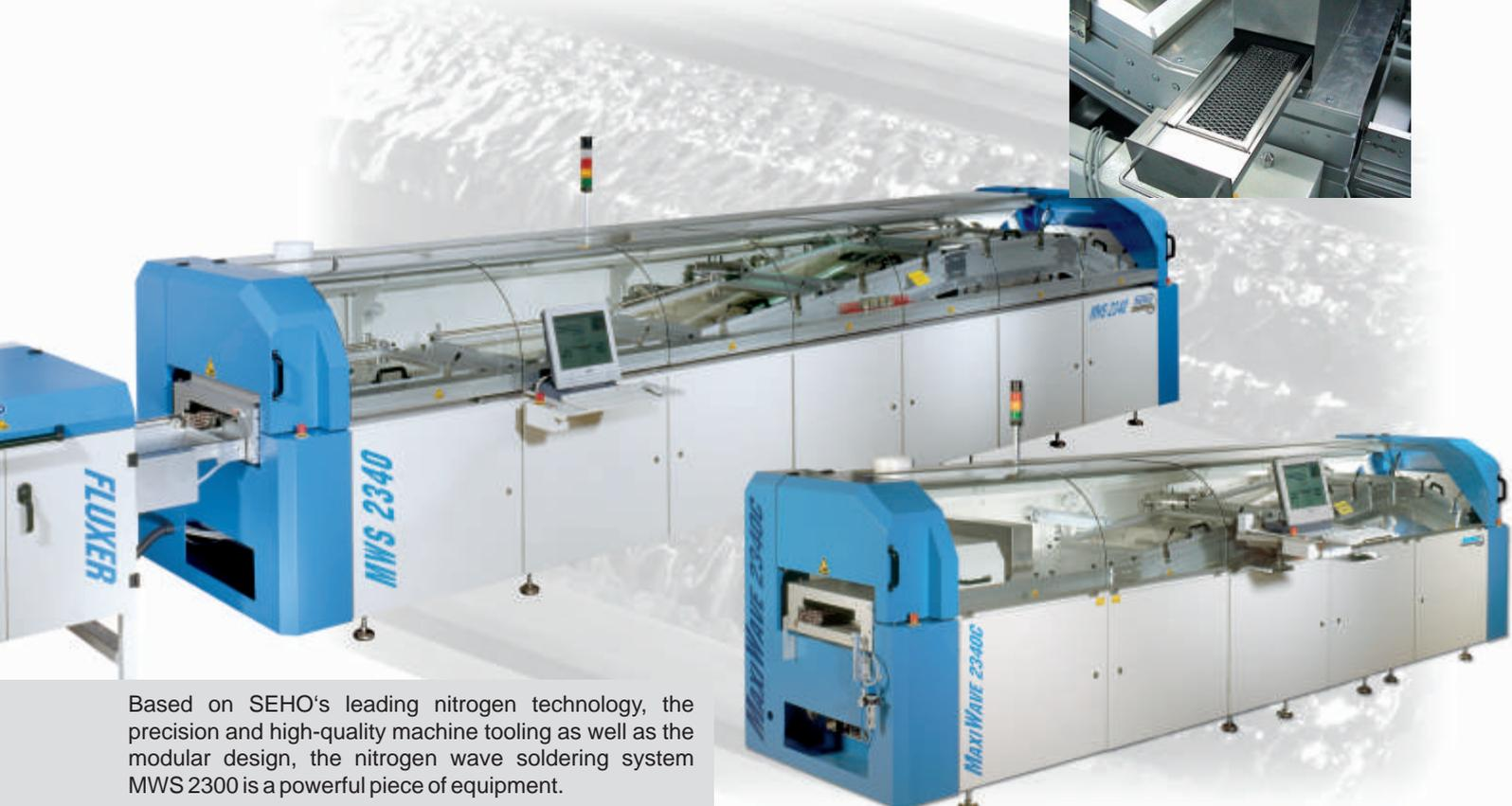
Based on SEHO's leading nitrogen technology, the precision and high-quality machine tooling as well as the modular design, the nitrogen wave soldering system MWS 2300 is a powerful piece of equipment.
